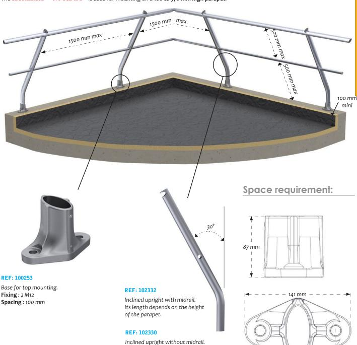
Its length depends on the height of the parapet (higher than 570mm).
